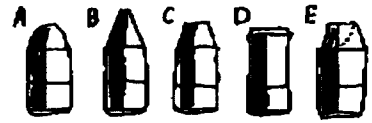
A few types of bullets: (A) Round Nose; (B) Spire point; (C) Semi-Wadcutter; (D) Wadcutter; (E) Hollow Point Semi-Wadcutter.
